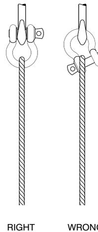
When a shackle is used to secure the top block of a set of wire rope blocks the load on this shackle is increased by the value of the hoisting effect.
