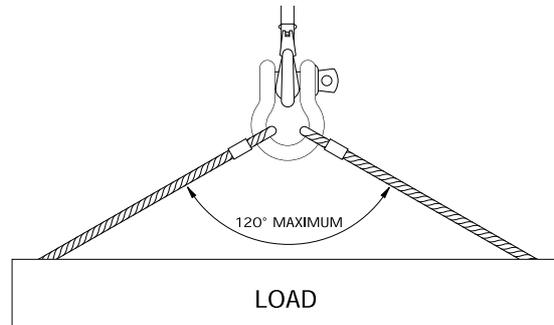
When a shackle is used to connect two slings to the hook of a lifting device, a bow type shackle must be assembled with the slings in the shackle body and the hook engaged with the shackle pin. The angle between the slings should not exceed 120°.
