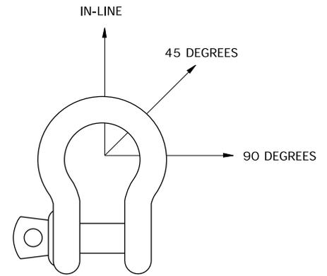
In-line loading is considered to be a load perpendicular to the pin and in the plane of the bow. Load angles in the table are the deviating angles from the in line loads.
